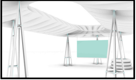
2. roof (inflatable, PVC)
